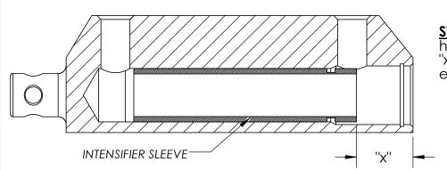
**STEP 1**: Without O-ring installed, insert intensifier sleeve into housing until firmly seated to determine length "x". Length "x" is determined by measuring the distance between the end of the intensifier sleeve and the end of the housing.
