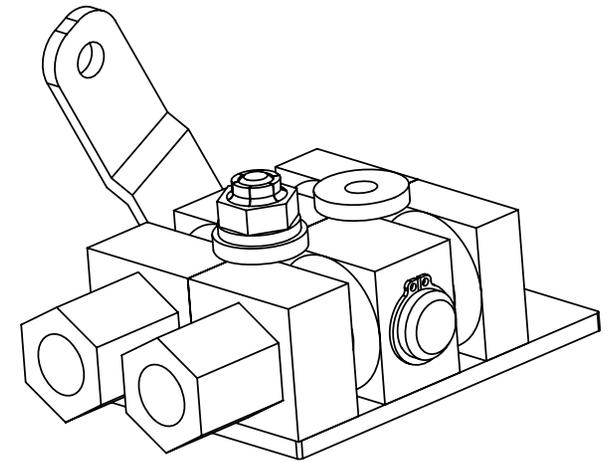
Installation Provides Same Alignment Between PV-1 Mount Holes and Cam Centerline
