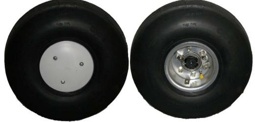
MATCO mfg announced the availability of a hub cap kit for the 5 inch MH series wheels today (such as MHE51B). Responding to customer inquiries for a kit to allow installation of the current WHLWC wheel cover on MH series wheels, MATCO mfg has introduced the MHWC hub cap kit.
