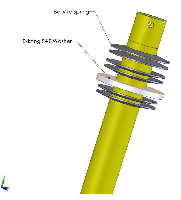
Use 3 Series Sets of Double Stacked Bellville Springs as Shown. Replace top Castle Nut with Thinner Slotted Jam Nut. Bottom Nut May Be Changed If Needed.
