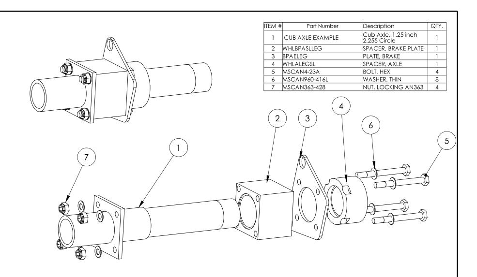
Axle is not part of kit and shown for assembly clarity only Items 2-7 in MHESL-CUBKIT. #3 is swapped for existing BPAE on Assembly This Kit also includes MHESLJ-KIT disc spacer kit to be installed on 'E' Seires wheel
