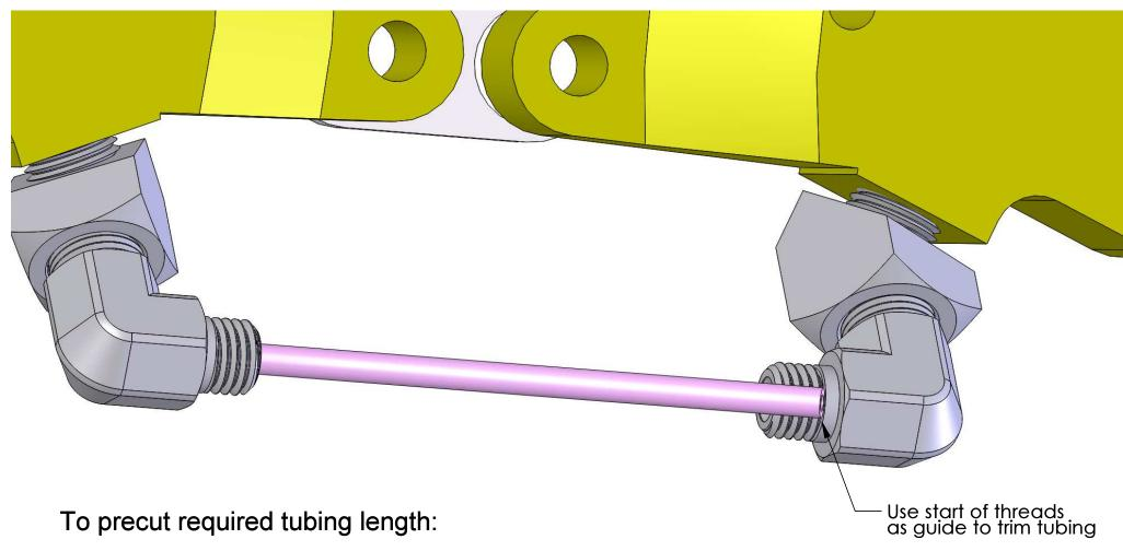
1) With nut and ferrules removed, insert one end of tubing fully into one fitting 2) Using fittings as a guide, trim opposite end of tubing even with start of threads on opposite fitting
